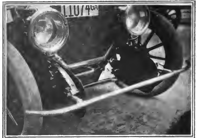
Fig. 13—Mud guards of this nature keep the radiator clean on long tours
